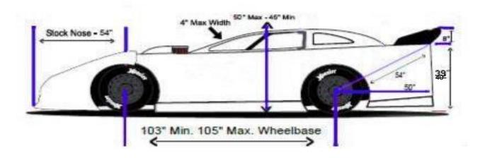
Rear deck height measured from ground to top of T-Bar is 40" with driver in car. The measurement of the spoiler is 8" from deck to top of spoiler.
